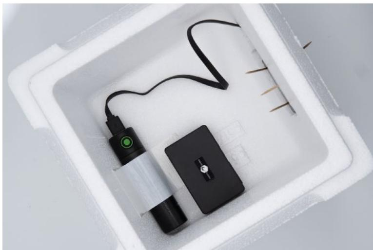
You can attach this to the bottom of the STRATOfinder and fix it to the bottom of the Styrofoam probe. Make sure that the Stratoflights logo on the top of the STRATOfinder is pointing towards the sky, as this is where the GPS antenna is located for optimum reception.
