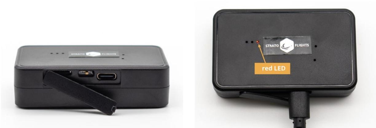
Now, carefully insert the provided USB-C cable into the port. Next, connect the USB cable to your computer or use your smartphone's USB charging adapter. Once the STRATOfinder is properly connected to the power source, please continue charging it until the red LED is no longer illuminated.
