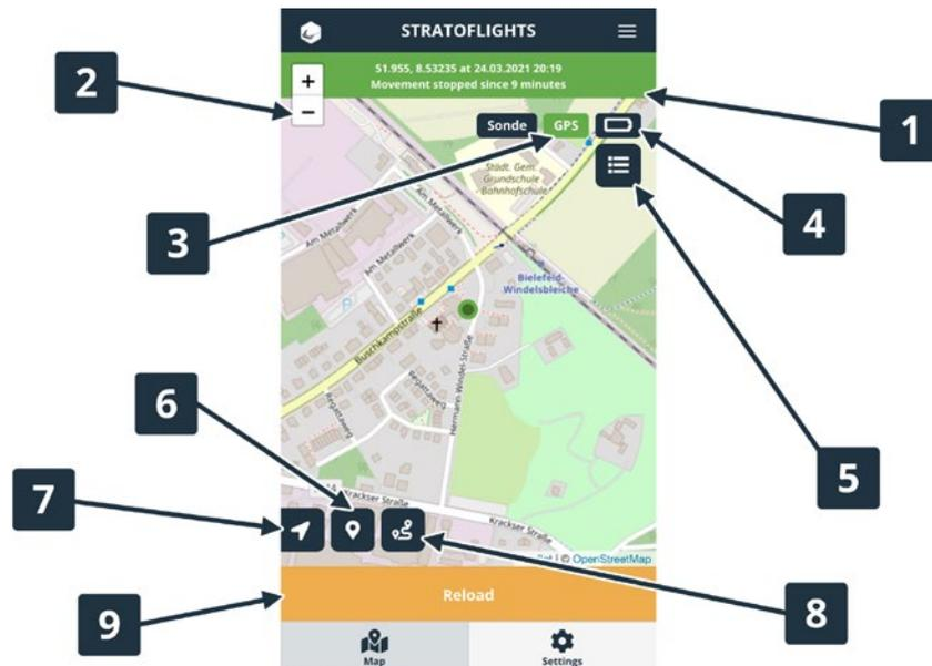
**1** In this green area, the position data is given in longitude and latitude and information is provided about the date and time at which the data was last sent and whether, for example, the „movement“ of the GPS tracker has been stopped. If the point no longer changes, the stratospheric probe has most likely landed at these coordinates.
