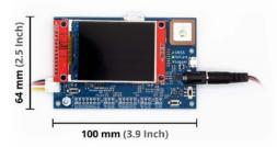
The battery-powered Datalogger STRATO4 measures and stores various data such as GPS coordinates, altitude, temperature, air pressure, humidity as well as UV radiation and light intensity.
