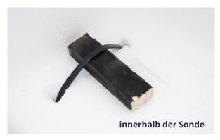
it cannot withstand much pressure. Please be careful with the cable ties and do not damage the Polystyrene probe. The supplied pieces of balsa wood sticks should be used on the other side of the cable ties to "balance" the pressure.
